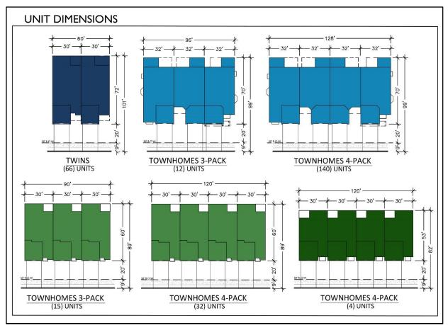
Concept Plan-Unit Dimensions Detail: Knickerbocker Tract
